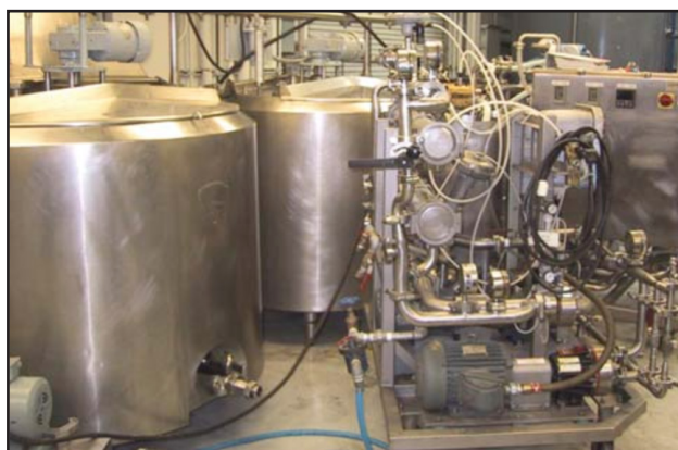
Figure 2: Jacketed stainless steel reaction tanks with 300-gallon capacity, also used as holding tanks
