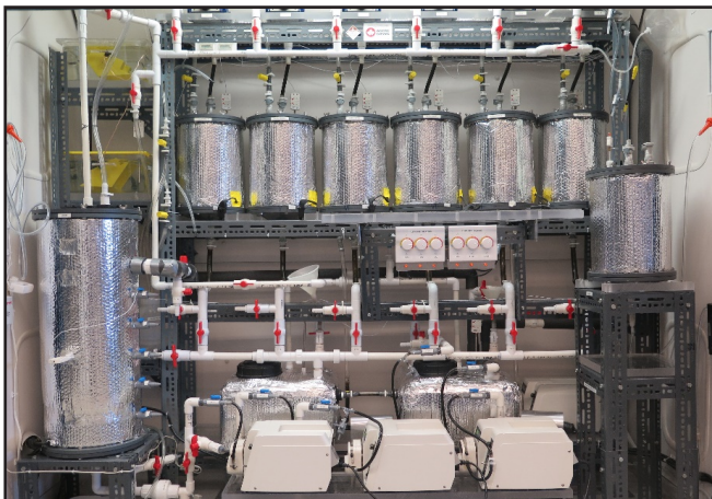
Figure 1: Two-stage anaerobic digester: sequentially-fed leach beds and an up-flow anaerobic sludge blanket reactor.
